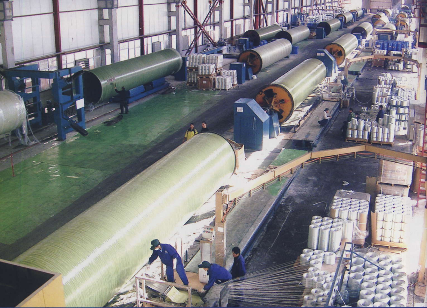
The Azkompozit factory has 15 computerised filament winders.
