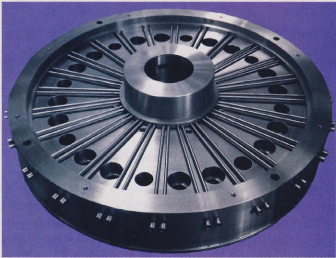
The Flexring system regulates individual multilayer blown film layer thicknesses with an online thickness measurement, monitoring and regulation system developed by IKV
